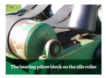
Belt tension can be changed by loosening the bearing pillow blocks on the idle roller see the picture to the left. Push the roller out and tighten. This will rise the bale on the turntable. It will also prevent the belt slipping when very heavy or light bales are being wrapped. Check film overlap after this adjustment.
