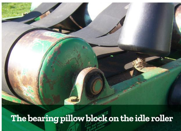
**The bearing pillow block on the idle roller**
